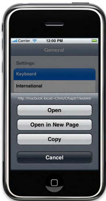
Figure 6–4. Touching and holding on elements such as links or images may trigger an option callout
