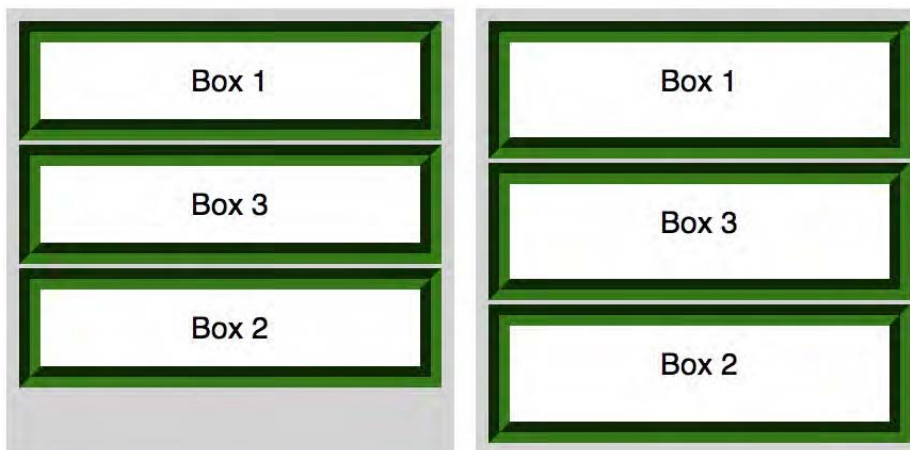
Figure 6-34. Layout with default box-flex value, which is (0.0), and box-flex set to 1.0
