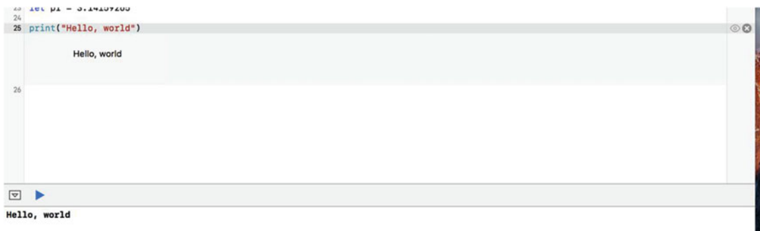
Figure A-4. Viewing output inline with the code and in the debug area
