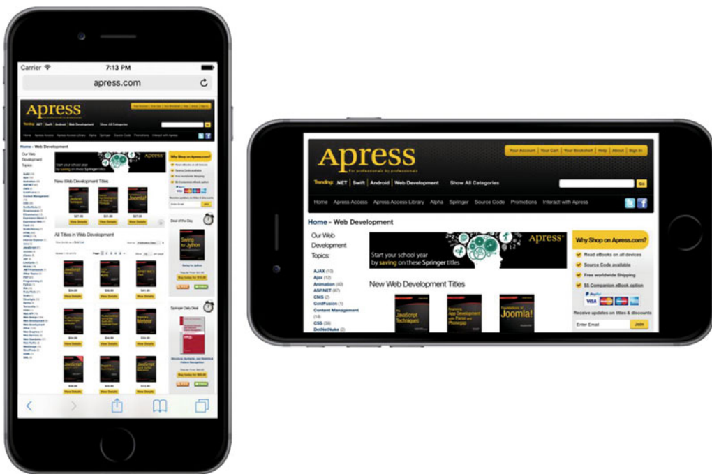
Figure 5-1. Like many iOS applications, Mobile Safari changes its display based on how it is held, making the most of the available screen space
