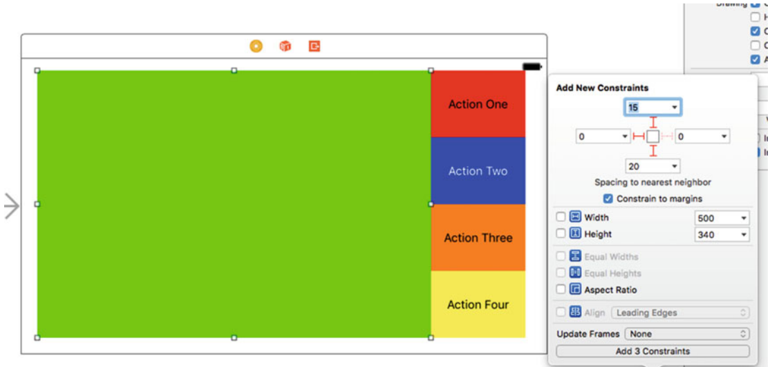
Figure 5-35. Pin the green view to the top, left, and right for the landscape orientation
