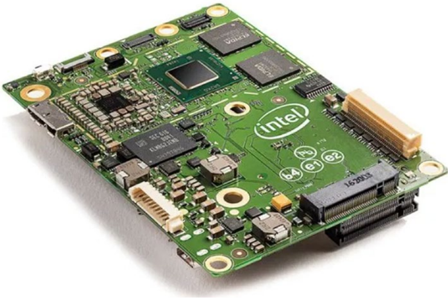
Figure 1-2. PCBA mounted with SOC and subsystems
