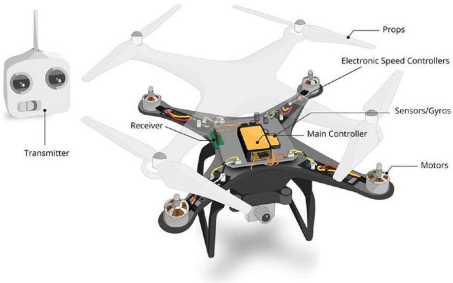
Figure 1-4. Parts of a drone
