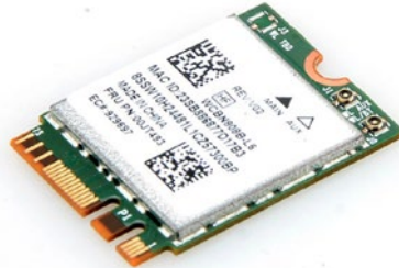
Figure 3-10. Integrated WiFi+BT module in a M.2 form factor
