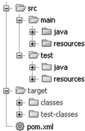
Figure 1-9. Standard Maven directory structure
