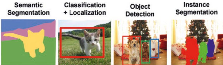
Figure 6-1. A visual explanation of the different terms describing the general task of locating one or more objects in an image
