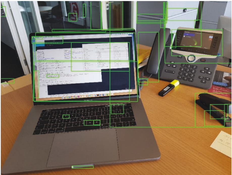
Figure 6-13. An example of the output of the selective search algorithm as implemented in the OpenCV library
