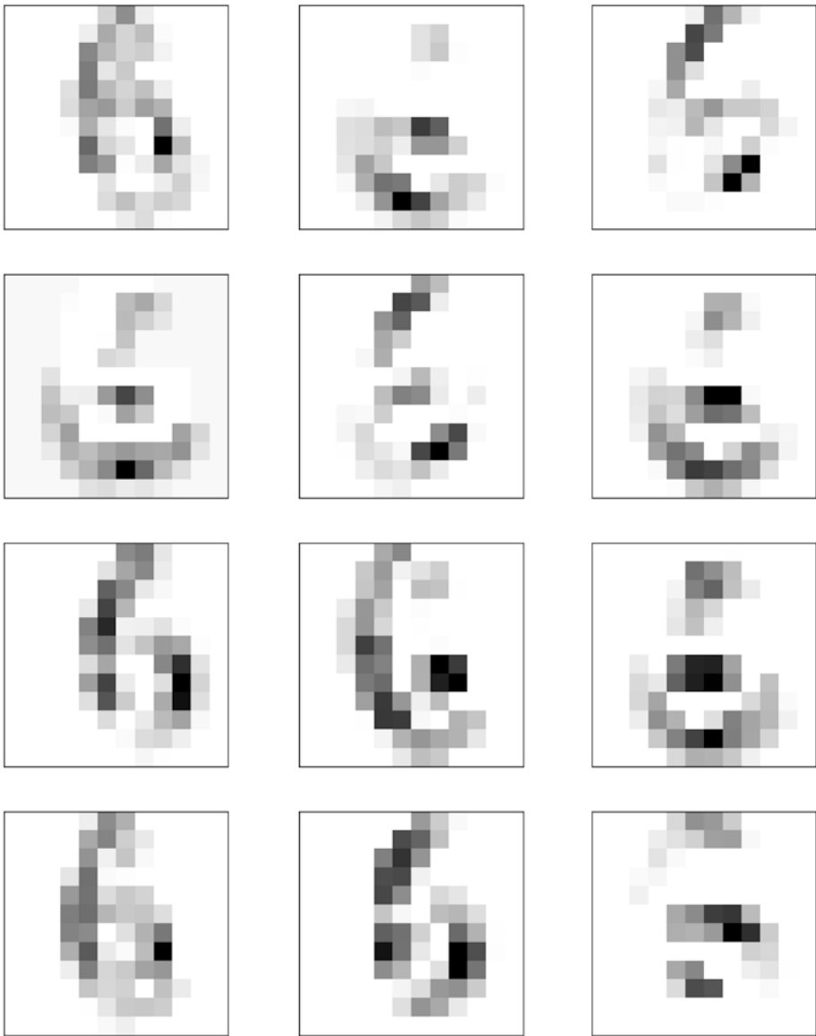
Figure 3-19. The output of the pooling layer when applied to the first 12 tensors coming from the convolutional layer
