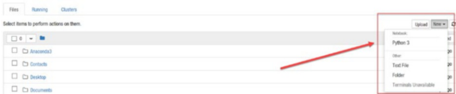
Figure 1-9. To create a new notebook, click on the New button located on the top-right part of the page and choose Python 3
