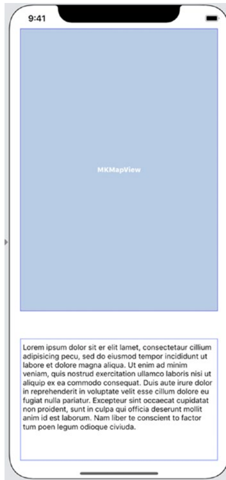
Figure 11-2. Placing a Map Kit View and a text view on the user interface
