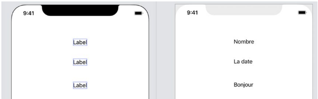
Figure 8-11. The preview pane showing French text defined in the Main.strings (French) file
