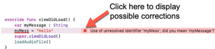
Figure 2-2. Syntax errors often keep a program from running, which allows Xcode to identify the syntax error
