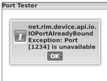
Figure 9-5: Your app receives this exception if it tries to listen on a port other code is using.
