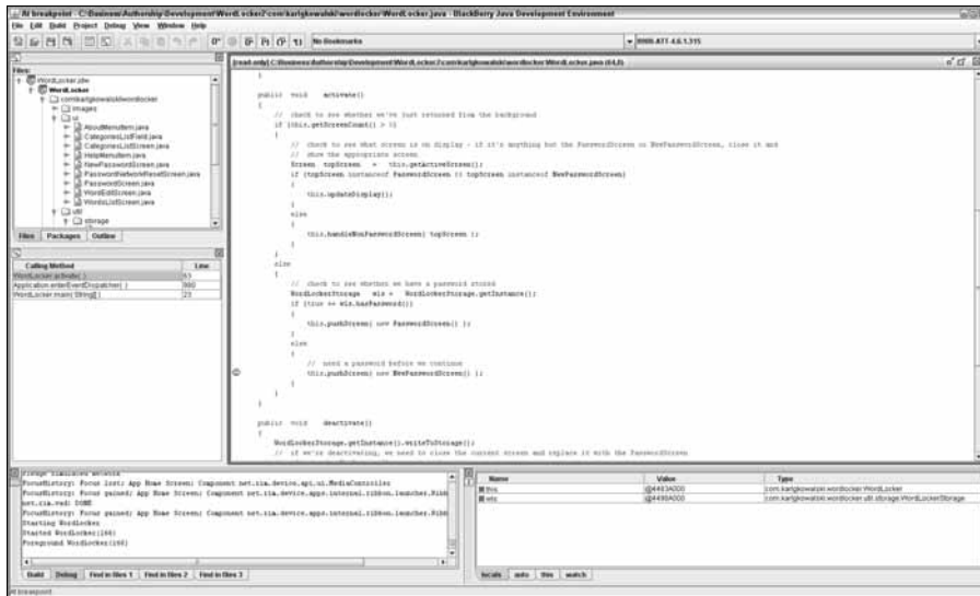
Figure 11-5: The Debugger stopped right before the New Password Screen object is pushed onto the screen stack.
