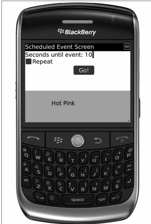
Figure 7-2: The layout manager places the custom UI class EventField at the bottom of the screen.
