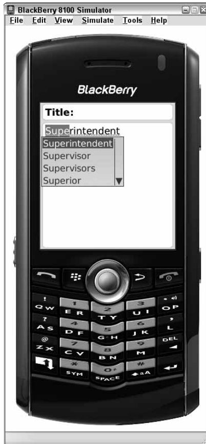
Figure 1-8: The BlackBerry Pearl and its SureType keyboard, with its guesses for the word I type.
