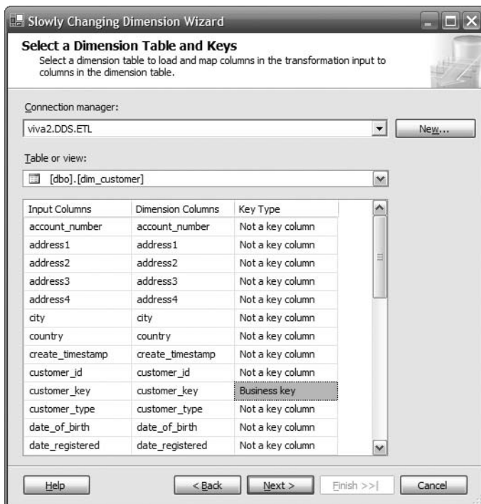
Figure 8-32. Mapping the columns of customer table on the Slowly Changing Dimension Wizard
