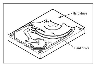
Figure 7-1: A run-of-the-mill hard disk drive.
