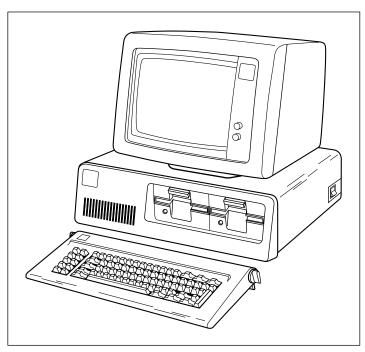
Figure 3-1: The original IBM PC.
