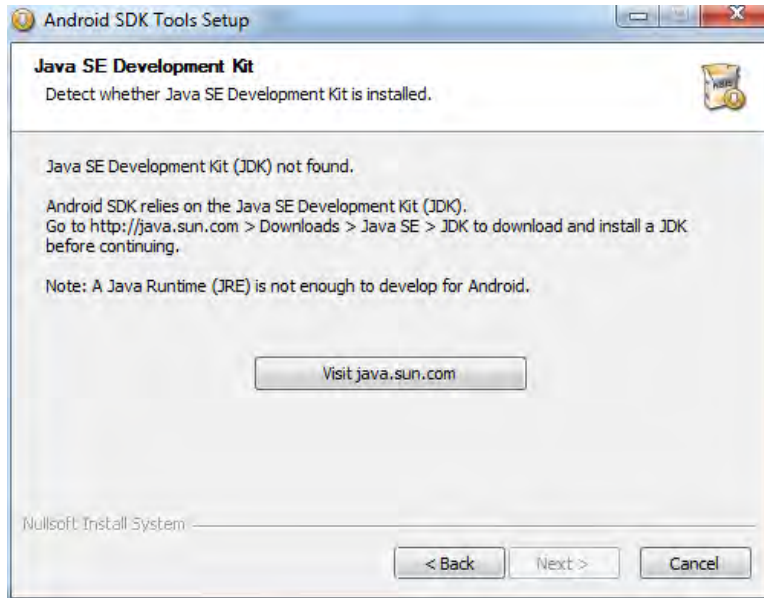
Figure 2-20. Missing JDK screen
