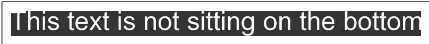
Figure 16-8. This text aligns to the top of the picture, as our code does, so that the baseline is no longer right at the bottom and the “g” is fully visible
