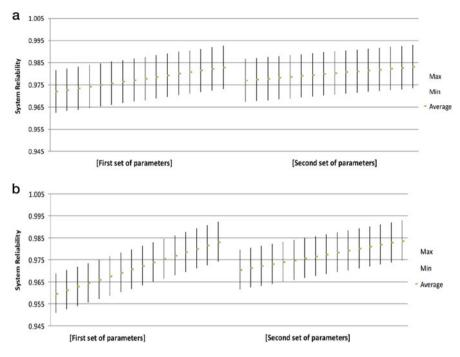
Fig. 14 System reliability obtained by embedding the reliability of an SCA-ASM component. (a) Considering the service  $s_3$  as an SCA-ASM component. (b) Considering the service  $s_7$  as an SCA-ASM component
