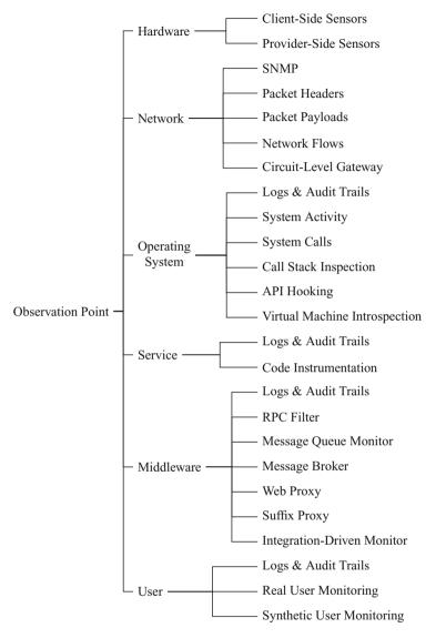
Fig. 4 An enumeration of potential observation points in client-cloud interaction monitoring
