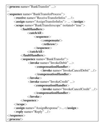
Fig. 19 The BPEL description of a redesigned BankTransfer process
