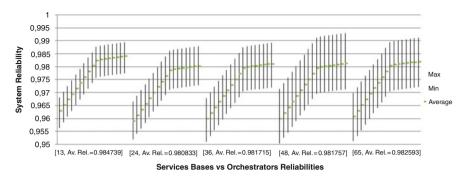
Fig. 11 System reliability obtained for the SCA assembly considering the orchestrator's reliabilities
