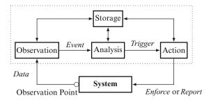
**Fig. 1** A monitoring system has four main components: observation, analysis, action, and storage. An observation point represents technical means to recognize a system's state and state changes. The observation component acquires data and generates *events*. The analysis component processes events and *triggers* the action component if necessary. The action component can then *enforce* actions or *report* events
