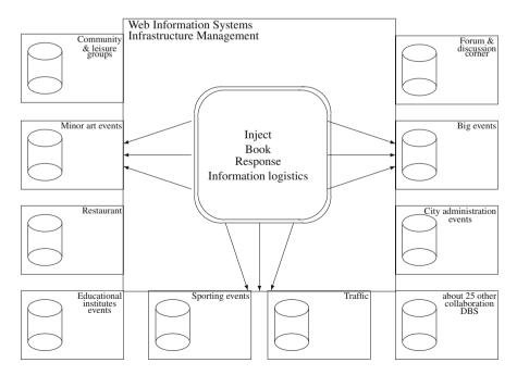
Fig. 7 The architecture of a database system providing views and functions for infotainment sites
