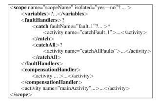
Fig. 11 A BPEL scope element containing fault and compensation handlers
