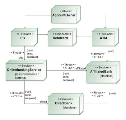
Fig. 2 Deployment diagram for the banking example
