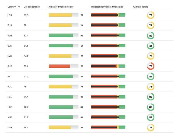
Figure 4-20. Linear Status Meter and Circular Status Meter examples
