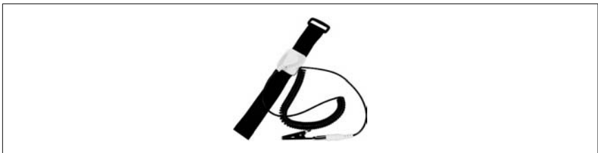
Figure 2-18. Antistatic wrist strap
