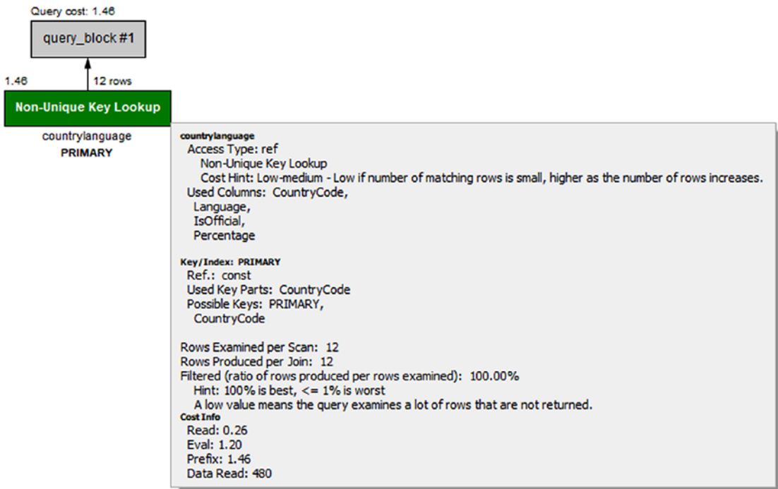
Figure 20-11. Visual Explain diagram for using part of a multicolumn index
