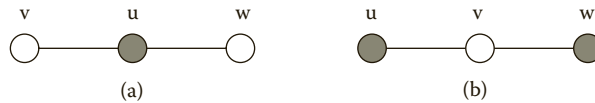
Figure 3.7 (a) Node u is in independent set. (b) Node u and node w are in independent set.
