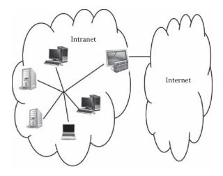
Figure 8.7 Firewall serving as a gatekeeper at the LAN's entry point.
