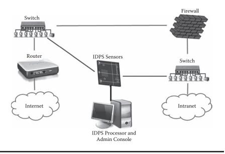
Figure 7.4 IDPS topology with passive sensing.
