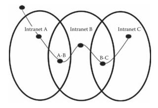
Figure 7.2 Intrusion from network A to network C via network B.
