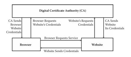
Figure 4.3 The principle of digital certificates.
