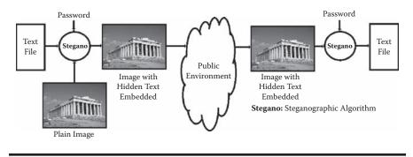
Figure 4.5 Principle of steganography. Text file hidden in an image.
