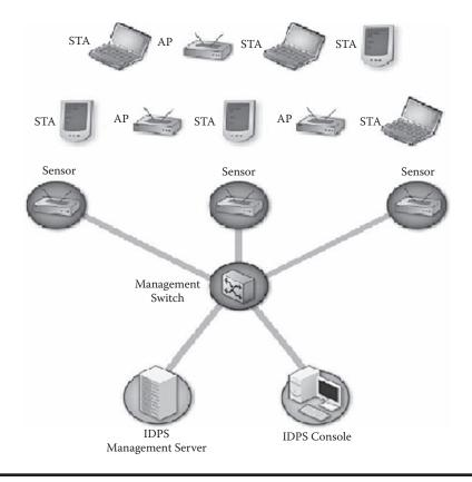
Figure 7.9 Typical configuration of a WLAN IDPS.
