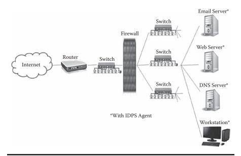
Figure 7.7 Typical configuration of a host-based IDPS. (From http://www.enterasys.com.)
