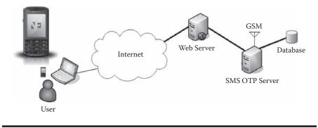
Figure 2.2 Authentication technology using an OTP delivered as an SMS to the user. (Courtesy of Nordic Edge, http://www.nordicedge.se.)
