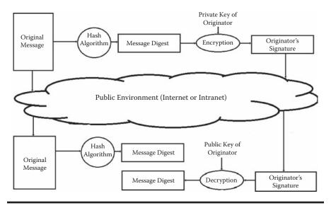
Figure 4.4 The principle of digital signatures.
