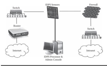
Figure 7.3 IDPS topology with in-line sensing.
