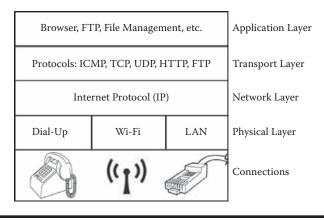
Figure 8.8 Layers hierarchy with typical content.
