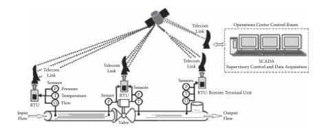
Figure 10.1 Remote Supervisory Control And Data Acquisition (SCADA) system [12].
