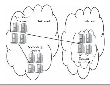
Figure 8.3 An advanced disaster recovery configuration. Courtesy of EXFO, Inc. [6].
