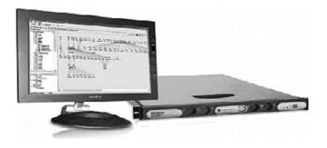
Figure 7.5 Administration control console of an appliance-based IDPS. Enterasys Dragon Network IDS Appliance (Fast Ethernet) [7].
