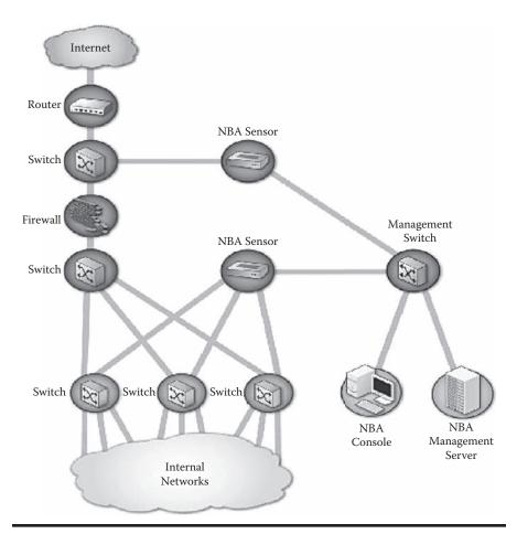
Figure 7.8 Topology of an NBA intrusion detection system. (From http://www.juniper.com.)
