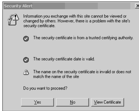
Figure 9-8 Browser Detecting Mismatch Between the Common Name and the Web Site Domain Name
