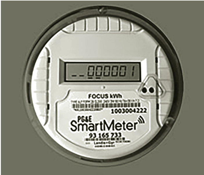
Figure 4.3 Smart meter example. (From PG&E, see http://www.pgecurrents.com/2012/06/12/pge-catches-wave-on-smartmeter-deployments/ .)
