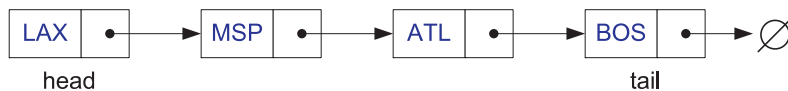
Figure 3.9: Example of a singly linked list of airport codes. The next pointers are shown as arrows. The null pointer is denoted by \emptyset .
