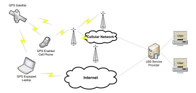
FIGURE 1.2: Mobile-based location provider architecture.
