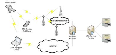
FIGURE 1.3: Location provider-based location provider architecture.
