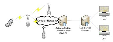
FIGURE 1.1: Network-based location provider architecture.
