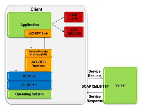
FIGURE 9.2: The entire process and components of the Web services API.
