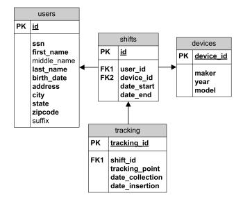
FIGURE 7.2: Design of the database of our LBIS tracking system example.
