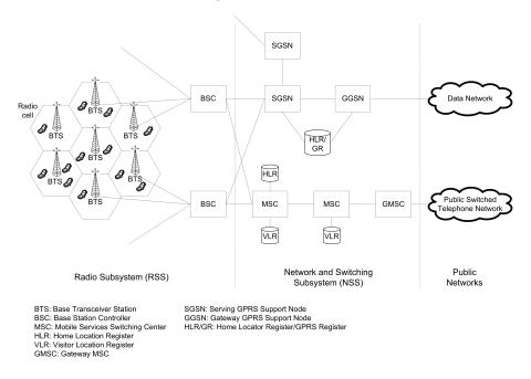
FIGURE 6.4: The GPRS cellular network architecture.
