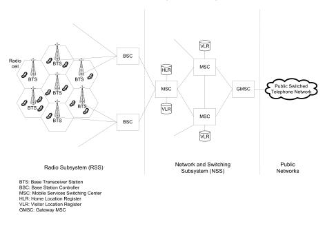
FIGURE 6.3: The GSM cellular network architecture.
