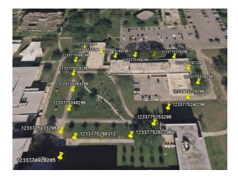
(b) Trip with the CPA algorithm. Only critical points are sent to the server.
