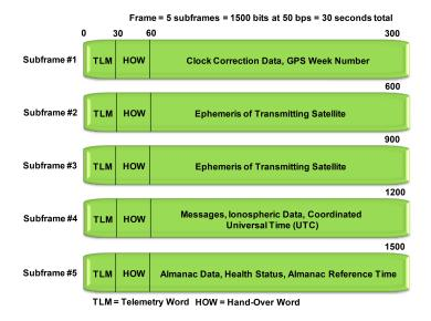
FIGURE 6.1: The GPS frame structure.
