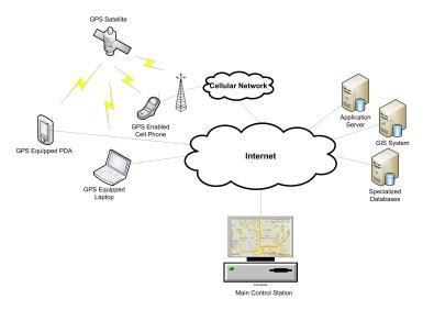
FIGURE 1.4: A complete LBIS real-time tracking system example.
