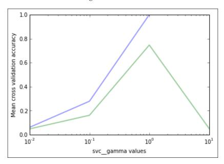
So the best result is for a gamma value of 1, where we obtain a training accuracy of 0.999 and a testing accuracy of 0.760.
