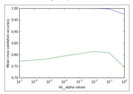
As expected, the training accuracy is always greater than the testing accuracy. We can see in the graph that the best testing accuracy is obtained with an alpha value in the range of  $10^{-2}$  and  $10^{-1}$ . Below this range, the classifier shows signs of overfitting (the training accuracy is high but the testing accuracy is lower than it could be). Above this range, the classifier shows signs of underfitting (accuracy on the training set is lower than it could be).
