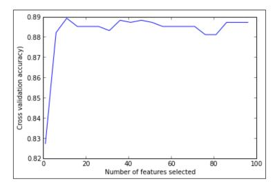
We can see that accuracy quickly improves when we start adding features, remaining stable after the percentile of features turns about 10. In fact, the best accuracy is achieved when using 64 of the original 581 features (at the 11 percent percentile). Let's see if this actually improved performance on the testing set.
