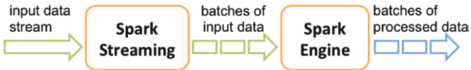
Figure 3-4. Spark Streaming batch processing
