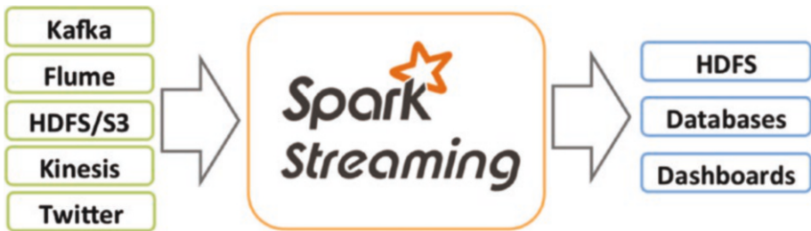
Figure 3-3. Spark Streaming data flow
