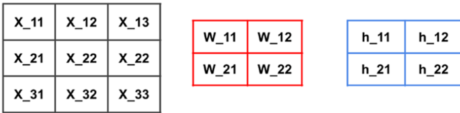
Figure 11-21. The input, weights, and output of the convolutional layer
