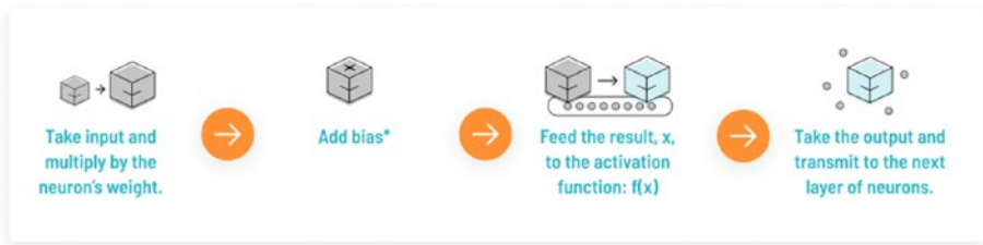
Figure 9-15. The steps of how activation works in a neuron
