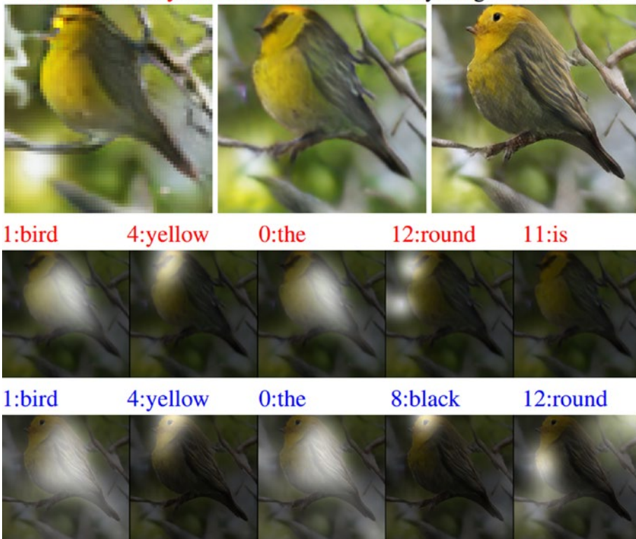
Figure 8-4. How an AttnGAN uses different parts of the text description to generate details for each region of the image
