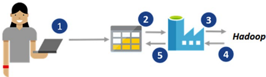
Figure 10-6. Example Databricks or HDInsight scenario: (1) Push videos to storage. (2) ADF reads the data from storage. (3) It calls HDInsight or Databricks to process the data. (4-5) The data are then streamed back and stored.
