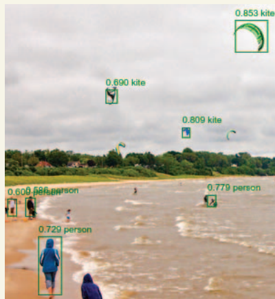
An example object-detection result from the TensorFlow.js version of the Single-Shot Detection (SSD) model. Notice the multiple bounding boxes and their associated object class and confidence scores.
