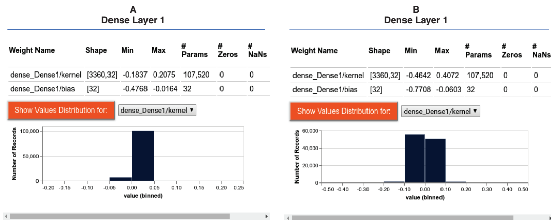
Figure 8.5 Distribution of the values in the kernel with (panel A) and without (panel B) L2 regularization. The visualization is created with tfvis.show_layer() . Note that the x-axes of the two histograms have different scales.
