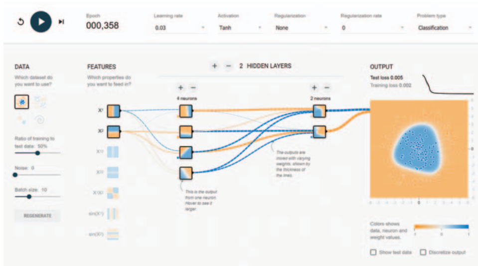
Figure 1.6 A screenshot of TensorFlow Playground ( https://playground.tensorflow.org ), a popular browser-based UI for teaching how neural networks work from Daniel Smilkov and his colleagues at Google. TensorFlow Playground was also an important precursor of the later TensorFlow.js project.
