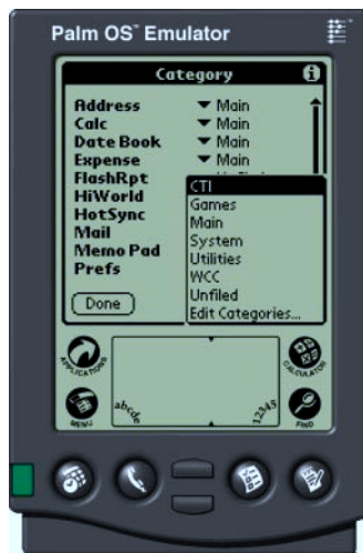
Figure 8.24 The category of any application, like HiSmallWorld, can be changed in the Category editor. Each application or database loaded on the device (or emulator) is displayed in a scrollable list. Next to each application is a dropdown list of categories. To change the category of an application, simply select another category from the dropdown list.
