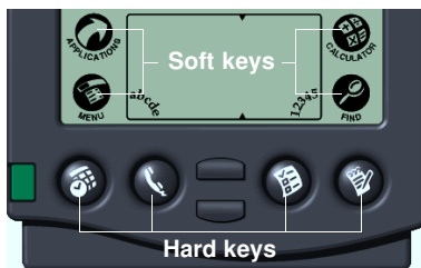
Figure 9.1 The Soft and Hard Keys on a Palm OS device allow for a user to quickly launch a Palm OS application such as the Calculator or Address Book. A Spotlet can be set up to be notified when one of these system keys is pushed.
