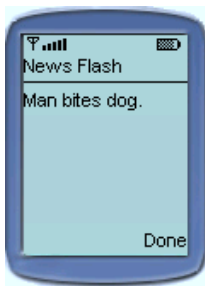
Figure 5.12 An alert works as a kind of message box in MIDP. Alerts can be used to provide warnings, information, error messages, etc.
