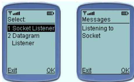
Figure 13.6 Running MsgListener for the first time. The MsgListener creates a StreamConnectionNotifier and waits for activity on the specified port.
