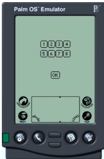
Figure 11.6 The combination lock example on Palm OS. This design allows a user to tap a sequence of buttons (1-8) to gain access to an application. This metaphor allows an application to be password-protected without burdening the user with character-based passwords. This design takes advantage of the pen-based user interface.
