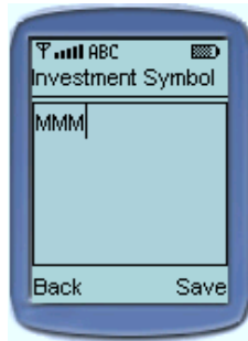
Figure 5.17 For user convenience, when text fields are selected or “entered” by the user, the device may offer a system-generated display for easier text entry. In the emulator, entering the symbol in the text field results in a system-generated display for capturing the symbol as shown here.
