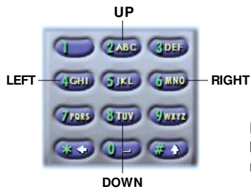
Figure 5.24 If the key pad does not have arrow keys, number keys must be used instead.
