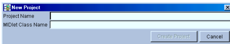
Figure D.3 A new project name and associated first MIDlet are entered in this window that displays after pushing the New Project... button on the KToolBar.
