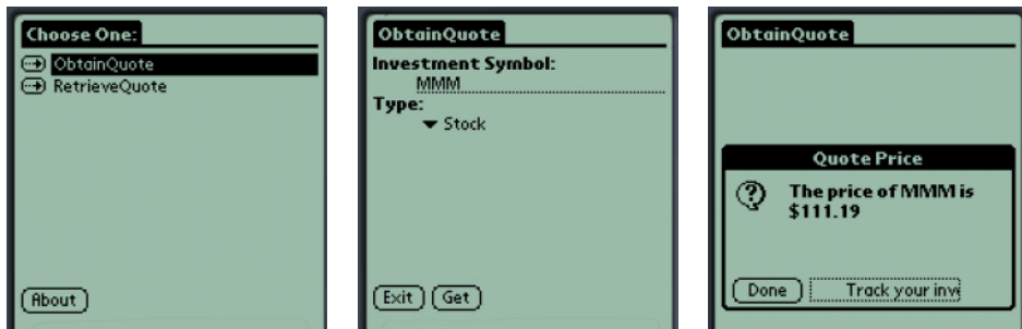
Figure 5.35 Running the ObtainQuote MIDlet in the Palm OS looks similar to running the MIDlet on the phone emulator. After selecting the QuoteMID... icon as seen in figure 5.34, a selection list allows the customer to select which MIDlet in the suite to run. The other two screens depict the EntryForm for entering the investment symbol and type and the Alert for displaying the investment price.
