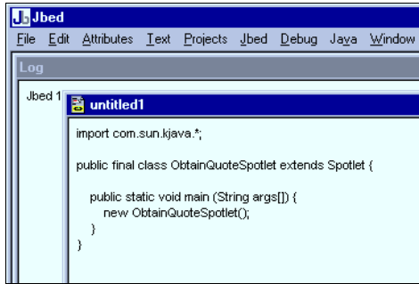
Figure 9.6 Upon opening a New Java file, an “untitled1” editing window will open in the Jbed IDE. Enter the ObtainQuoteSpotlet code in the editor provided.
