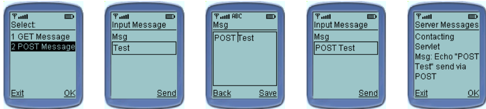
Figure 12.2 Running the EnterpriseClient application to perform a POST request. First the user selects “POST Message” from the main menu. Then the user enters a message to send and invokes the Send operation. The message is sent using an HTTP POST method and the response from the server is displayed.
