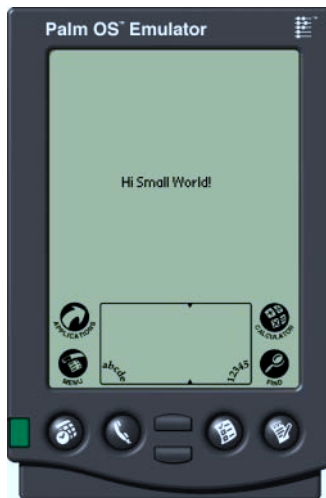
Figure 8.26 The HiSmallWorld application running on the emulator after successfully compiling, linking and deploying the HiSmallWorld.prc file to the emulator and tapping on the HiSmallWorld application icon.
