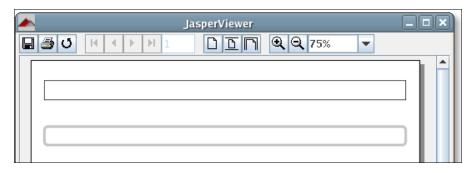
Notice how the line outlining the second rectangle is thicker than the first one. This is because we used the <graphicElement> subelement of the <rectangle> element. Like every text element can contain a subelement called <textElement>, every graphic element can also contain a subelement called <graphicElement>.
