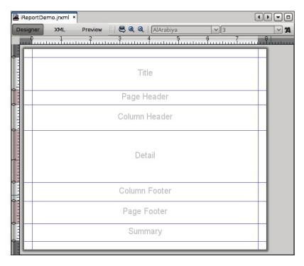
The horizontal lines divide the different report sections. Any item we insert between any two horizontal lines will be placed in the appropriate report section's band. Horizontal lines can be dragged to resize the appropriate section(s). The vertical lines represent the left and right report margins. It is not possible to drag the vertical lines. To modify the left and right margins, we must select the report in the **Report Inspector** window at the top left.
