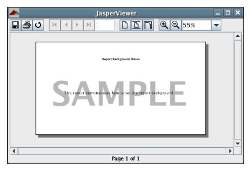
Notice how the background text appears to be behind the text in the <band> element.
