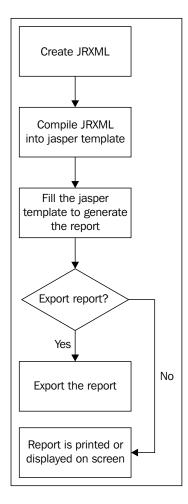
When working with JasperReports, the first step is to create a report template as an XML file. XML report templates can be handcoded or generated by a graphical report designer. Even though JasperReports report templates are XML files, by convention template filenames are given an extension of .jrxml. JasperReports XML templates are commonly referred to as JRXML files, which is the term we will use in this book.
