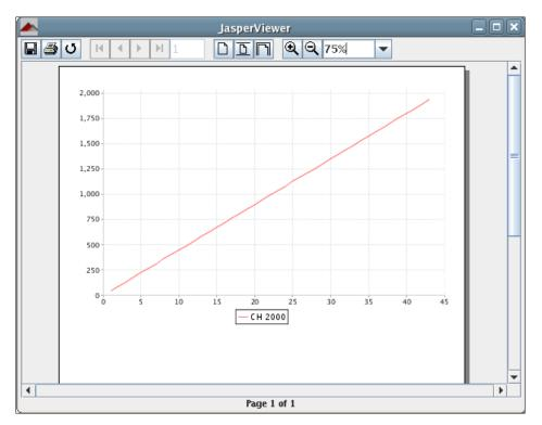
As we can see in the example, for XY line charts, the <dataset> element must be inside an <xyDataset> element and this element has no attributes. In addition to the <dataset> element, <xyDataset> may contain one or more <xySeries> element.
