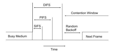
Fig. 4.2 Timing of 802.11 between two transmissions
