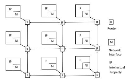
Fig. 8.2 A 2D  $3 \times 3$  mesh network
