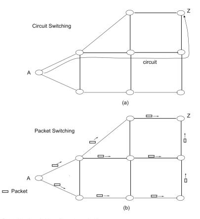
Fig. 1.5 (a) Circuit switching, (b) packet switching
