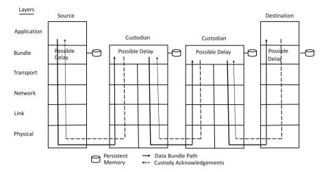
Fig. 9.4 Bundle protocol layered architecture
