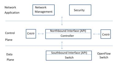
Fig. 7.3 Software-defined network architecture
