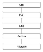
The protocol layers for SONET go by the names of path, line, section, and photonic (see Fig. 6.2 where ATM is being carried over SONET). The functions of the layers are [104]:
