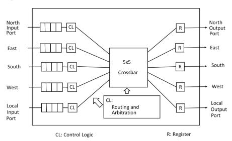
Fig. 8.3 Internal router structure for mesh node
