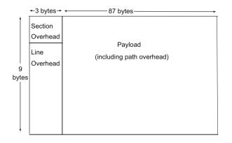
Fig. 6.3 An STS-1/OC-1 SONET frame with overhead indicated
