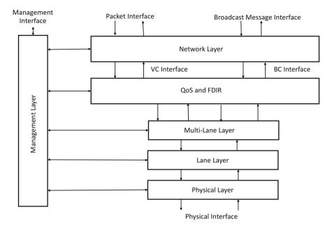
Fig. 9.3 SpaceFibre protocol stack
