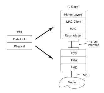
Fig. 2.4 Protocol stack for 10 Gbps Ethernet
