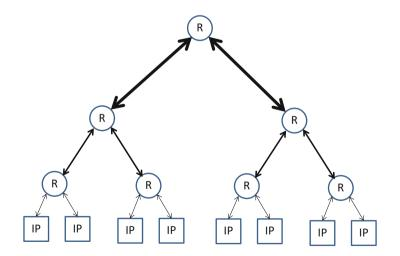
Fig. 8.5 Fat tree topology with routers (R) and intellectual property cores (IP)
