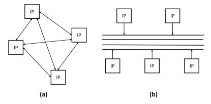
Fig. 8.1 Classic interconnection networks: (a) point-to-point interconnection and (b) bus inter-
