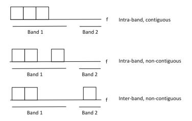
Fig. 4.3 LTE Advanced carrier aggregation modes
