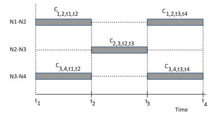
Fig. 9.6 Polar satellite model and contact timing diagram representation
