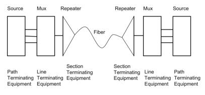
Fig. 6.4 SONET system diagram
