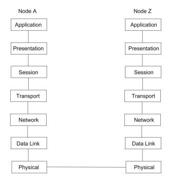
Fig. 1.6 OSI protocol stack for a communicating source and destination
