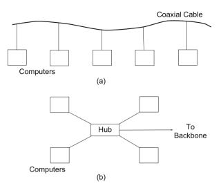
Fig. 2.1 Ethernet wiring using (a) coaxial cable and (b) hub topology
