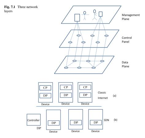
Fig. 7.2 (a) Classic and (b) SDN network architectures. Here CP is control plane and DP is data plane
