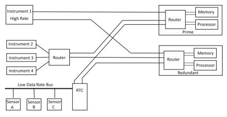
Fig. 9.2 More SpaceWire architectural features: data concentration
