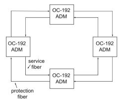
Typically, rings are implemented with multiple service and protection fibers (see Fig. 6.6). If a service fiber path fails, a protection (backup) fiber is switched on its place. The number of protection fibers can be less than the number of service fibers if one is willing to live with less redundancy. Also, if all of the fibers between two adjacent nodes are lost, with a sufficient number of protection fiber rerouting can keep a logical ring in place until repairs are made.
