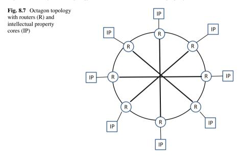
Finally another interconnection network that has been suggested for NOC use is the octagon topology (Fig. 8.7). There are 8 IP cores, 8 routers, and 12 two-way links. There are thus, at worse, two hops between any pair of routers. Each router requires a  $4 \times 4$  crossbar (one connection to the local IP core and three connections to other routers). Simple algorithms can yield fast and efficient shortest path routing [150]. Octagons can be connected together to form larger networks.
