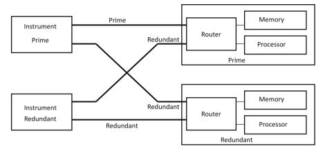
Fig. 9.1 Instruments and two data handling units
