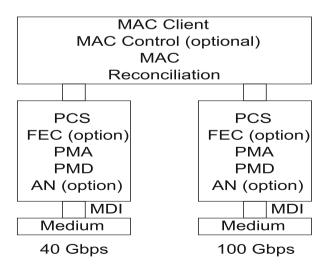
Fig. 2.5 40 and 100 Gbps Ethernet protocol functions
