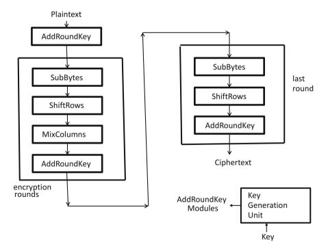
Fig. 11.1 AES encryption structure
