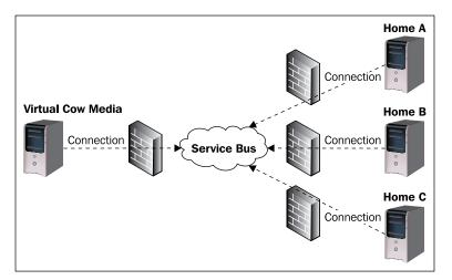
This outlines the use of the Service Bus as the message broker for all communication between the endpoints. As each of the endpoints connect to the Service Bus, a secured, tunneled connection is established. This is all accomplished in the cloud with few changes to existing code. Let us take a closer look at this solution in the next section.
