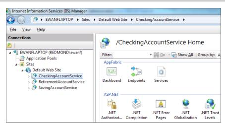
12. To verify that all services have been installed correctly using the appropriate **Application Pools** and are running the right version of the framework (should be 4.0), click on **Default Web Site**. Then in the main window under AppFabric, double-click on **Services**. This is shown in the following screenshot:
