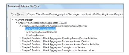
13. As we have a project reference and access to the data contracts assembly, our generated classes use these types. This enables us to pass the currentCustomer object to each of the backend service-request operations as an input variable. This is one of the advantages of having a shared data contracts assembly. We can also create some variables of type Account to represent the responses. Now create the following variables, by clicking on the AccountAggregatorScope first:
