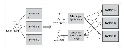
They could consider integrating the frontend application to all required backend systems, but this would dramatically increase the complexity of the application and if any other systems needed to connect to the same systems, that logic would need to be duplicated and maintained.
