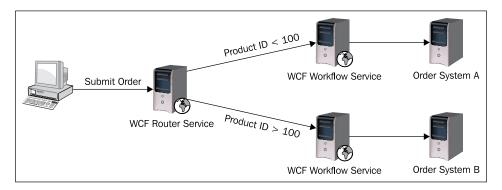
An order comes from a customer to a single endpoint at McKeever Technologies. This single endpoint then routes the order based on the content of the order (that is, the value of the Product ID element). The router sends requests to WCF Workflow Services, which can provide us durability and persistence when talking to the backend order management systems. If an order system is down, then the workflow gets suspended and will be capable of resuming once the system comes back online.
