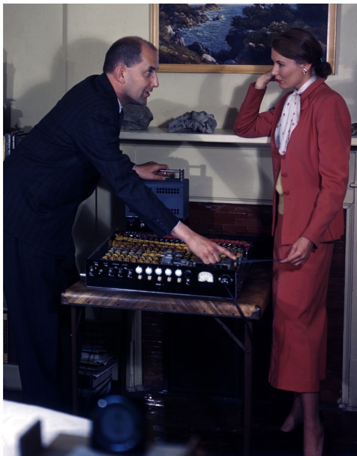
Berkeley explains how Simon gets instructions from a piece of punched tape. See Radio-Electronics , October 1950.
