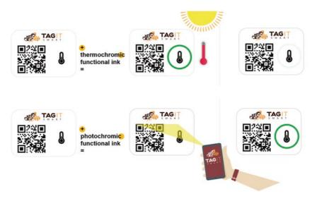
Fig. 4.4 Temperature and light sensitive smart tags
