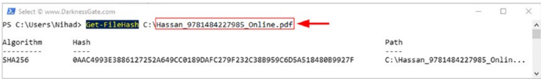
Figure 2-5. Using Windows PowerShell to calculate a digital file’s hash
