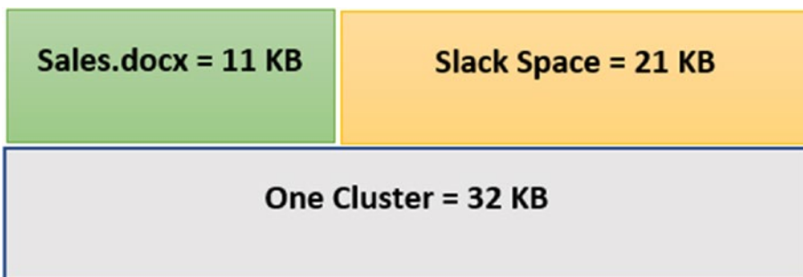
Figure 2-7. One cluster can hold only one file at a time
