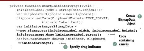
All we needed to do in this example was create a BitmapData object that had the same dimensions as the drag initiator (1), draw a copy of the drag initiator (the containing canvas in this case) in the BitmapData object (2), and then specify that object as the third parameter for the doDrag() method (3). The BitmapData object is then automatically applied as the drag indicator, and it follows the mouse wherever it goes, even outside the AIR application.
