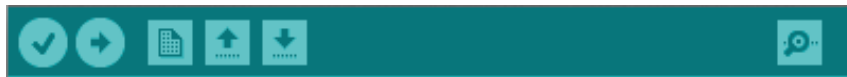
The Serial Monitor icon at the right most part of the Arduino toolbar
