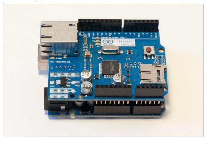
This is an image of the assembled board and the Ethernet shield:
