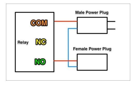
First, connect one pin of the female power plug to the **COM** pin. Then, connect one pin of the male power plug to the **NO** pin. Finally, connect the two remaining cables together, for example, using a typical electrical screw terminal.
