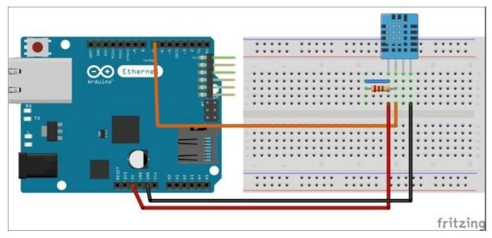
First, plug the DHT11 sensor to the breadboard. Then, connect pin number 1 and 2 of the sensor using the 4.7k ohm resistor.
