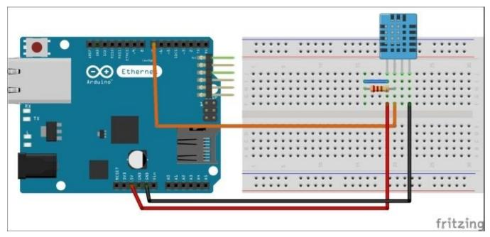
First, plug the DHT11 sensor into the breadboard. Then, connect the pin number 1 and 2 of the sensor using the 4.7k ohm resistor.
