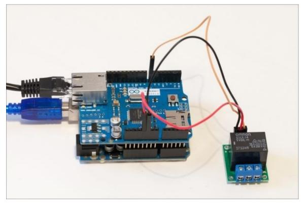
Then, you need to connect the power cables to the relay module. A relay module basically has three output pins: **COM** (for the common pin), **NC** (for the normally closed pin), and **NO** (for the normally open pin).
