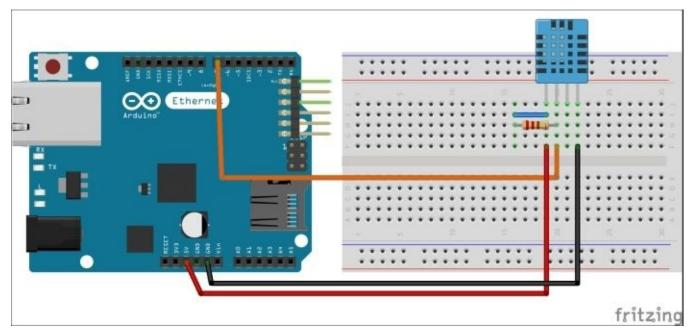
First, plug the DHT11 sensor to the breadboard. Then, connect pin numbers 1 and 2 of the sensor using the 4.7k ohm resistor.
