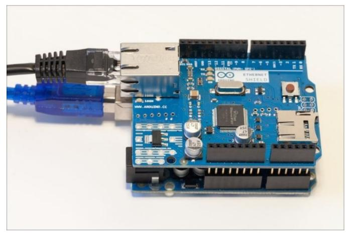
If everything is wired correctly, you should see the **ON** LED on the Ethernet shield is switched on, as well as the **LINK** LED near the Ethernet port.
