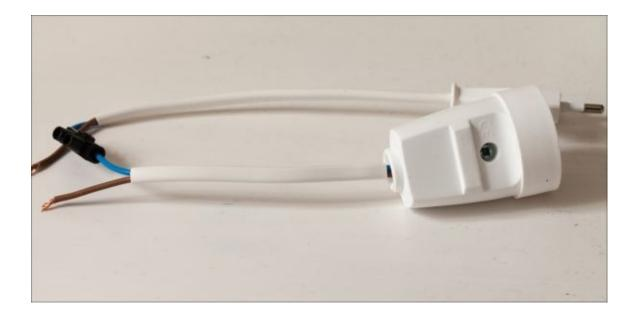
The male plug will be used to connect the relay to the main power plug in the wall and the female socket will be used to connect the device to control the relay.
