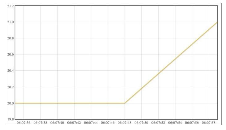
To illustrate the behavior of the sensor on the plot, I pinched it with my fingers and released it a bit later. As expected, the temperature went up before going down again after a while. The following screenshot is the result on the web page:
