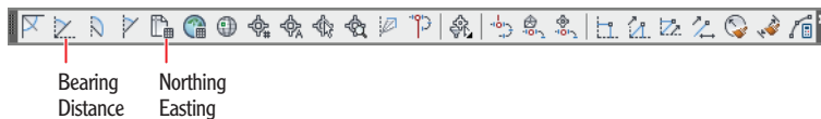
FIGURE 1.11 The Transparent Commands toolbar with red lines pointing to the Bearing Distance and Northing Easting transparent commands
