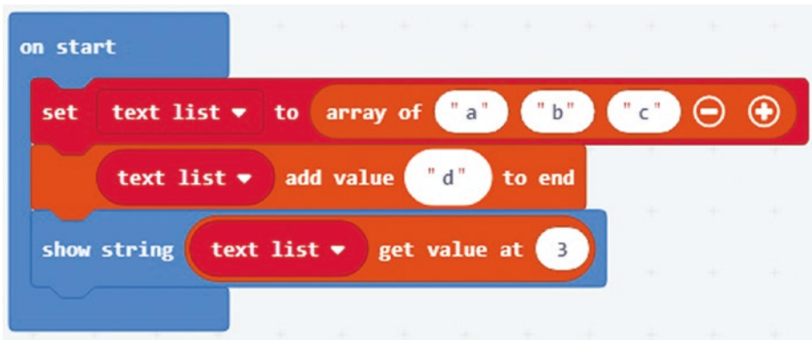
Figure 10-23. Inserting an item to the end of an array followed by verifying
