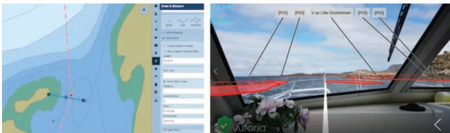
FIGURE 8.7 A very narrow passage on the test track. The distance between the 1-m shoal and the small skerry is 33 m (in the chart, left). Right, the app view entering the narrows (northbound). (Photo courtesy of the author.)
