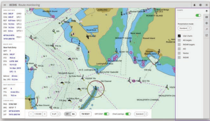
FIGURE 10.5 Electronic chart display and information system (ECDIS) main functions separated into interactive functions (right side) and information elements (left side).
