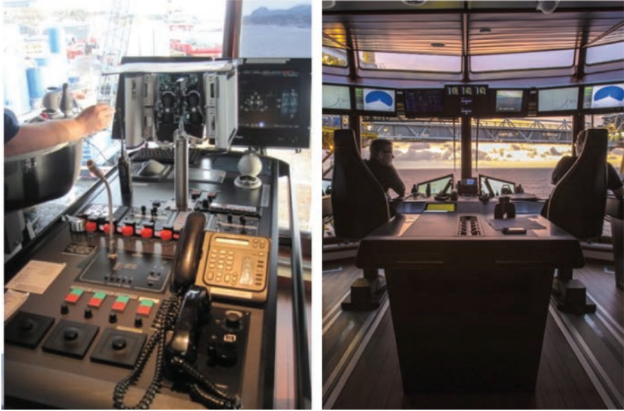
FIGURE 9.2 Illustration of pre-redesign (to the left) and post redesign (to the right) of aft bridge workstation.
