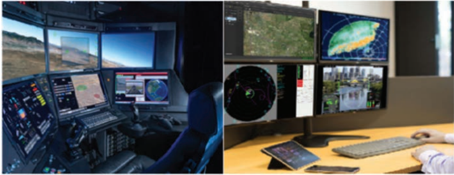
FIGURE 13.2 Cockpit paradigm (left), computer workstation paradigm (right) for GCS.
