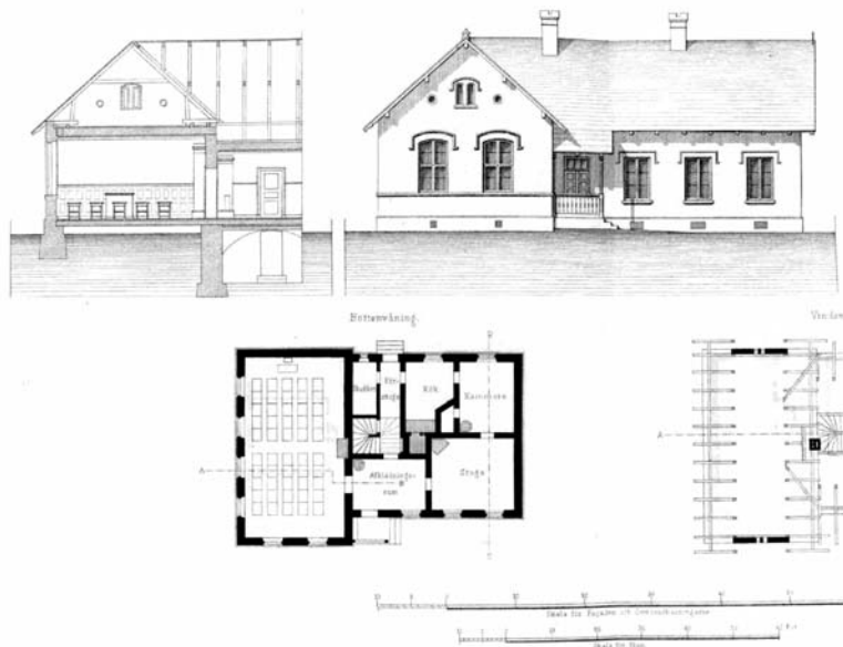
Figure 3.2 Sample design for a village school, 1865. We see the classroom, a room that separated indoors from outdoors for taking off outdoor clothes, and the teacher's lodgings, with a separate entrance, two rooms, kitchen, and pantry. From Normalritningar till folkskolebyggnader jemte beskrifning [Standard guidelines for elementary school buildings] (1865) (Stockholm: Öfverintendentsemetet), Uppsala University Library.
