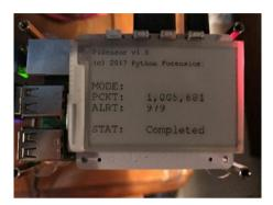
Figure 5-2. Raspberry Pi with PaPirus ePaper display
