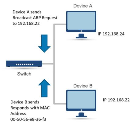
Figure 2-4. Simplified ARP request/replay process
