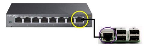
Figure 5-5. Connecting the Pi sensor to the TP-LINK monitoring port
