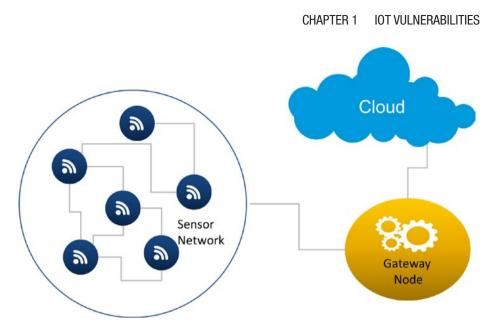
Figure 1-4. Device-to-gateway framework
