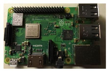
Figure 6-1. Raspberry Pi 3 Model B+
