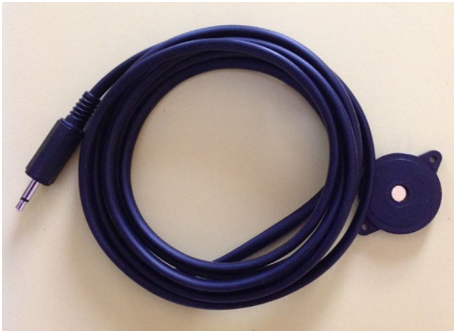
Figure 7-26. Piezo element wired to a 1/8-inch jack
