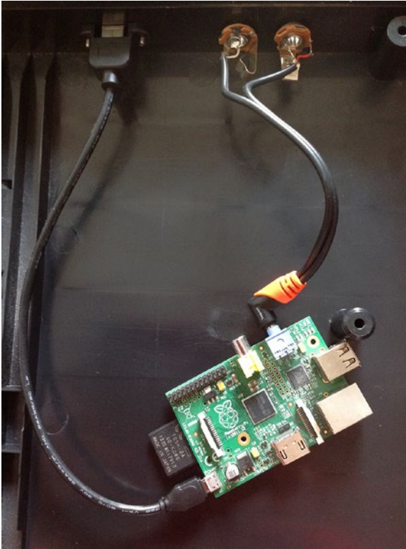
Figure 5-42. Getting the power input and audio output of the Pi outside the enclosure
