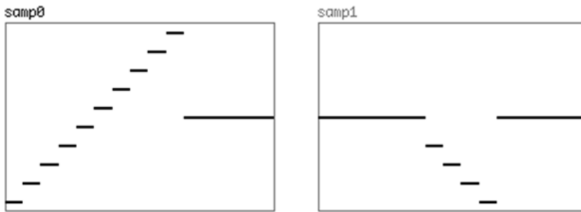
Figure 9-24. Copying samples 3 to 0 of samp0 to the indexes 6 to 9 of samp1
