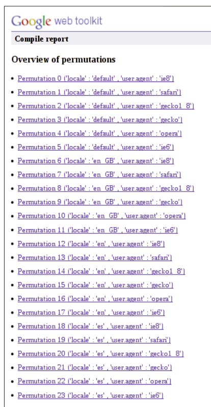
Figure 15.2 The basic compile report shows all permutations that were generated by the compilation process. The permutation numbers match those shown in Figure 15.1 but might vary.
