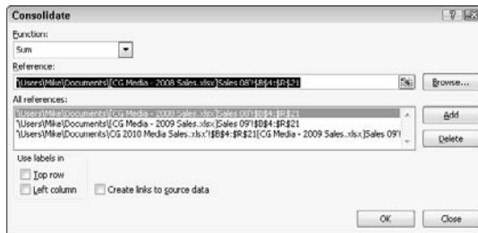
Figure 4-13: Using the Consolidate dialog box to total sales data for three years stored on separate worksheets.
