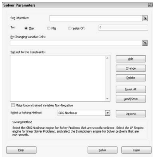
Figure 1-13: Specifying the parameters to apply to the model in the Solver Parameters dialog box.
