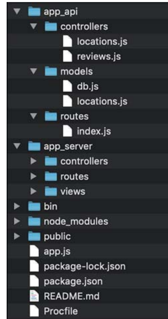
Figure 6.4 Folder structure of the application at this point. app_api has models , controllers , and routes , and app_server has views , controllers , and routes .
