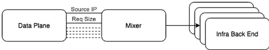
Figure 3-7. Data plane sending attributes to the attribute processor or Mixer
